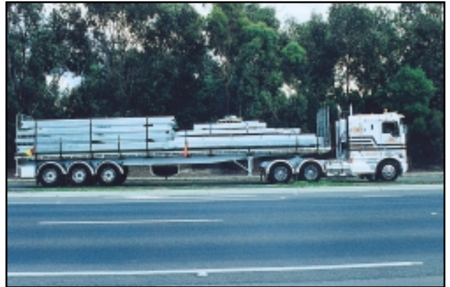
Carrying more than one overwidth item within the general length, height and mass limits
